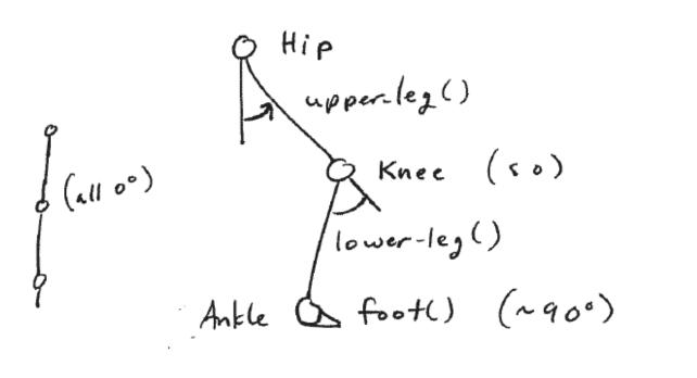
rotate (Hip, 0,0,1) upper-leg() ratate (Knee, 0,0,1) lower-leg rotate (Andrik, 0,0,1)  $f_{00}+()$
